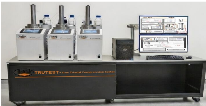
Three-pump assembly and computerised control & acquisition station
