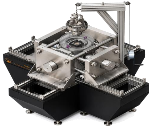
TRUTEST-C true triaxial load frame — four servo-controlled hydraulic actuators around the confining pressure cell
