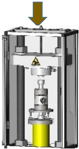
HOEK cell with strain gauges
