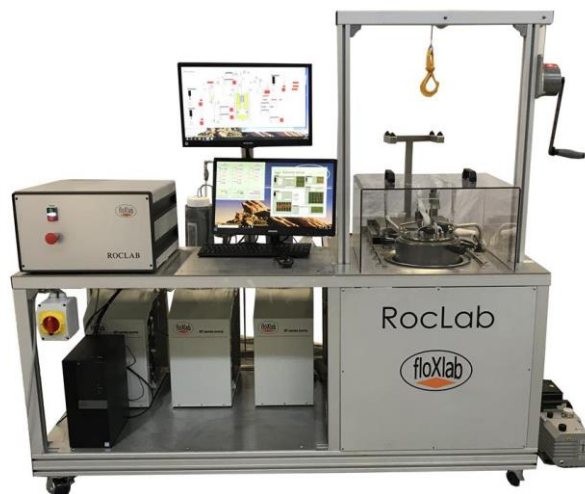
ROCLAB — Automated reservoir-condition compressibility test bench
