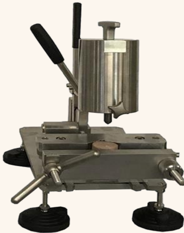
Cerchar Original — fully mechanical hard-rock abrasivity tester
