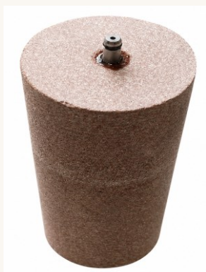
Specimen with axial borehole
