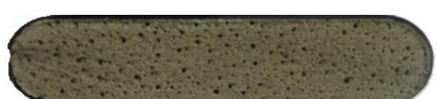
Slab face after acid etching
